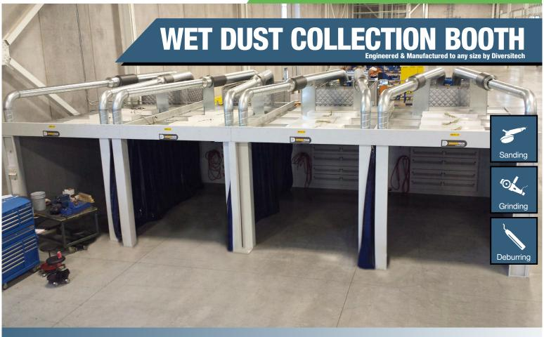
Diversitech's Wet Dust Collection Booth offers a simple, customizable and turnkey solution to handle combustible dust collection for larger work pieces. The stainless steel Wet Dust Collectors serve as the booth's filtration system, and range in size from 3000CFM, 5000CFM, and 6500CFM units. A standard auto-level water control system works to reduce maintenance and increase your production uptime
